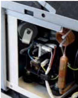
Step 5: Chek atau ganti kapasitor Start relay, overload switch.
